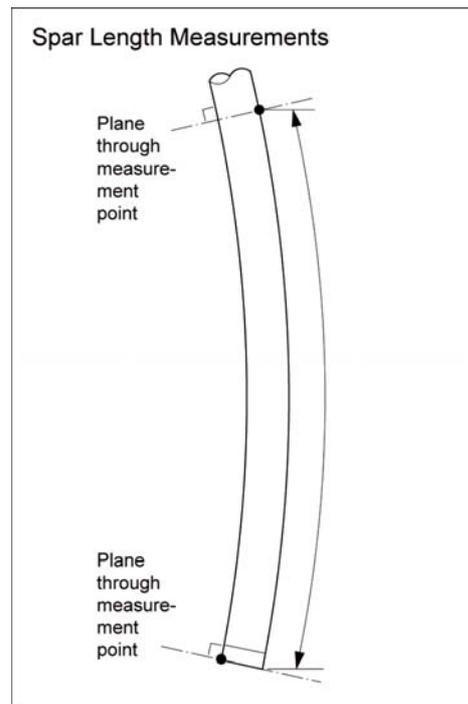
**H.4.2** Fittings, local curvature and local cut away, shall be ignored when measuring a **spar** or dimensions taken to a **spar**.
